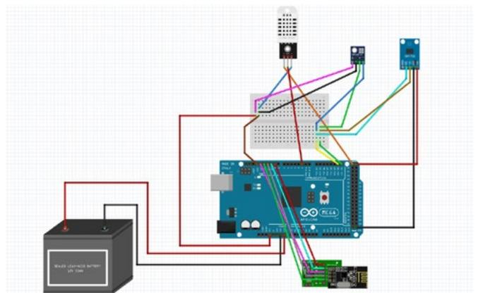
Figure 5. Sensor circuit diagram of transmitter side
