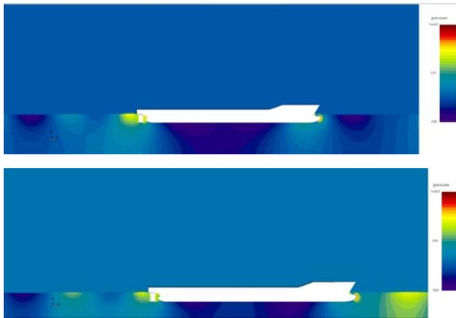
**Fig. 9** Pressure profile around the ship in shallow water ((upper:  $H=5T$ , lower:  $H=3T$ ))
