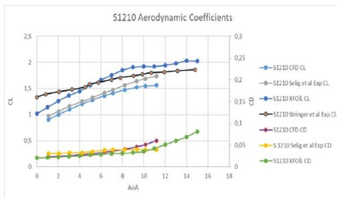
**Figure 6:**  $C_L$  and  $C_D$  values at different angles of attack ( $Re=1 \times 10^5$ ).
