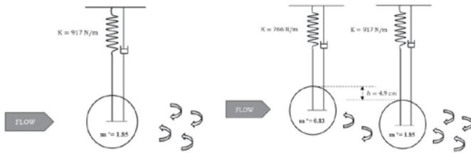
**Figure 2.** Schematic View of the Single Cylinder (Left). Schematic View of the Tandem Cylinders (Right)
