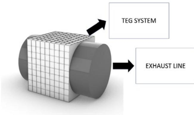
**Figure 2.** Integration of the TEG system into the exhaust line.
