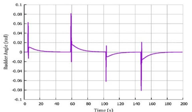
**Figure 4.** Rudder angle time history during the HIL simulation.
