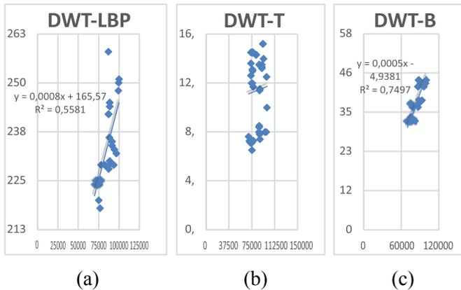
**Figure 2** Plotted DWT-LOA (a) DWT-T (b) and DWT-B (c)
