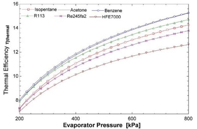
**Figure 2.** The effect of evaporator pressure on the thermal efficiency of the ORC (ORC) system for different ORC working fluid types
