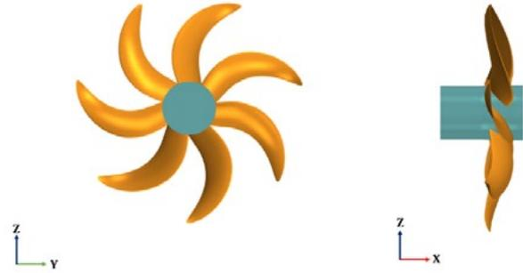
**Figure 2.** 3-D view of INSEAN E1619 Propeller
