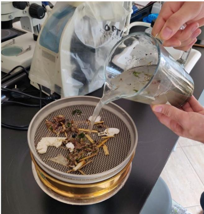
**Figure 10.** Sieving the sample through meshes of 2 different sizes
