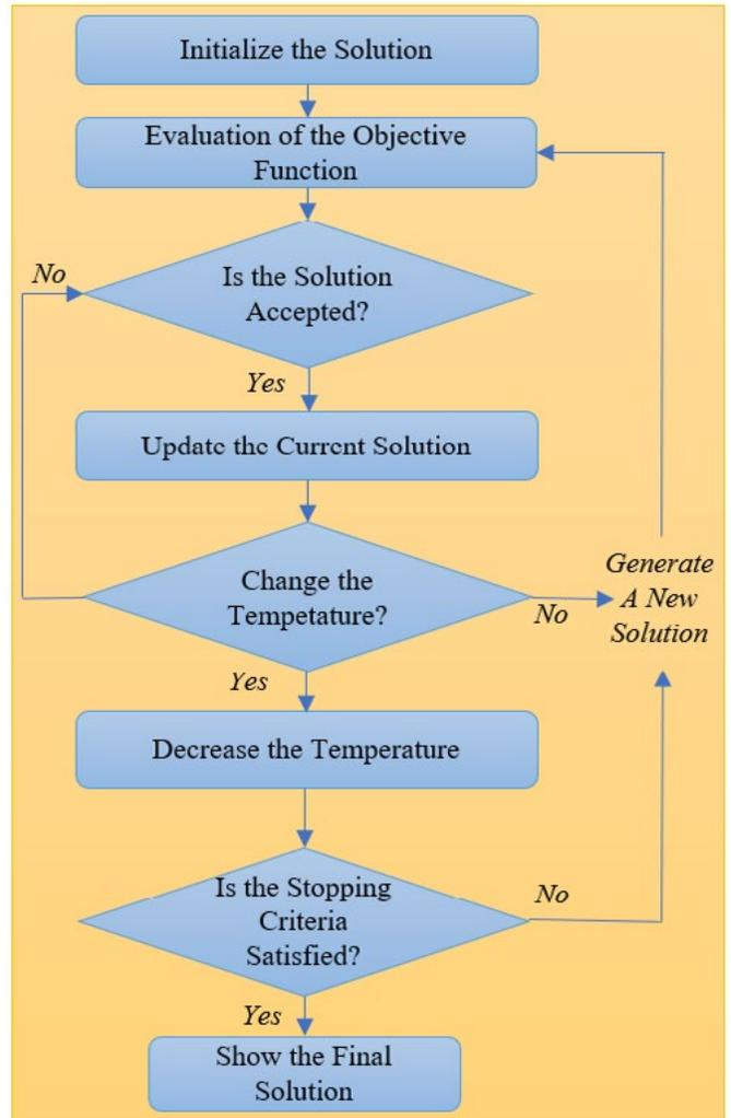
**Figure 6.** Flowchart of the Simulated Annealing Algorithm
