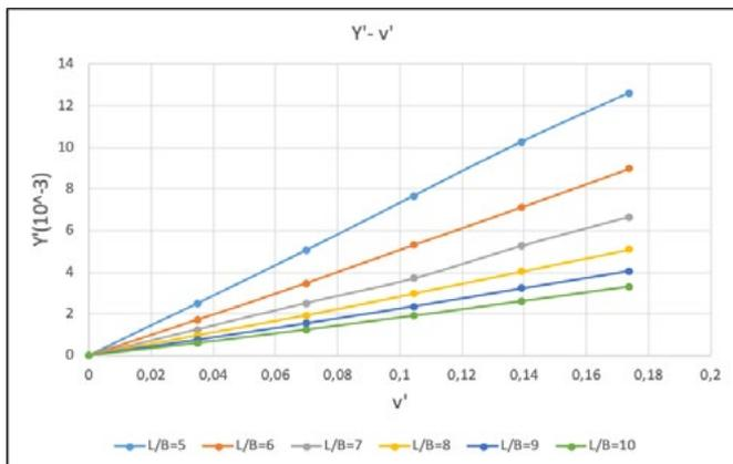
**Figure 13.** The Variation of Lateral Forces and Drift Velocities for Different L/B Ratios.
