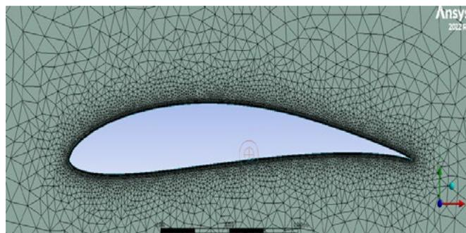
**Figure 4:** Mesh structure and boundary layer around foil section.
