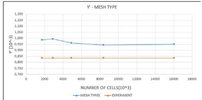
**Figure 6.** Displacement force (Y') for 2° static drift.
