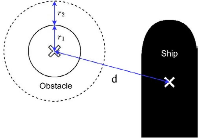
**Figure 6.** Safety parameter constrained by obstacle
