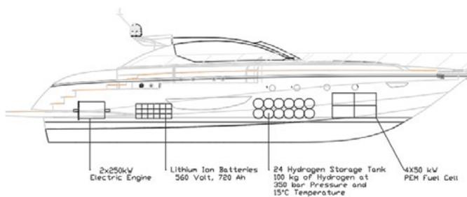
**Figure 3.** Schematic diagram of yacht propulsion system
