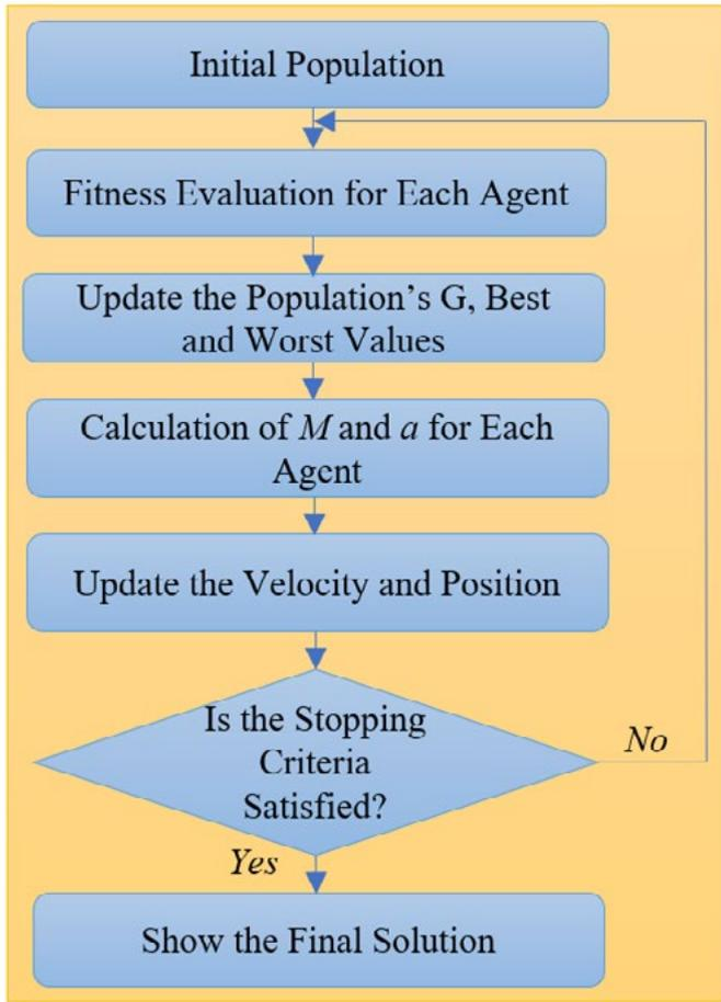
Figure 7. Flowchart of the Gravitational Search Algorithm
