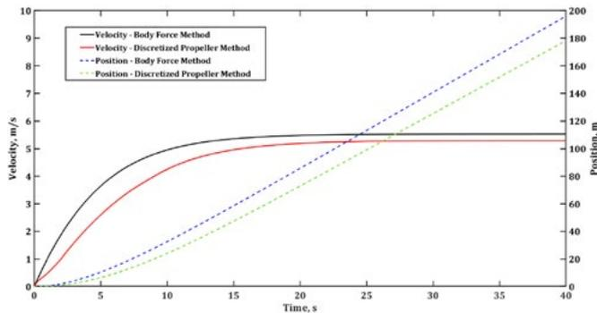
**Figure 10.** Comparison of the effect of the propulsion model on the submarine velocity and trajectory
