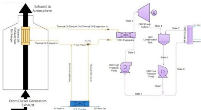
Figure 1. Model of ORC system for the marine vessel
