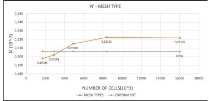
**Figure 5.** Yaw moment (N') for 2° static drift.
