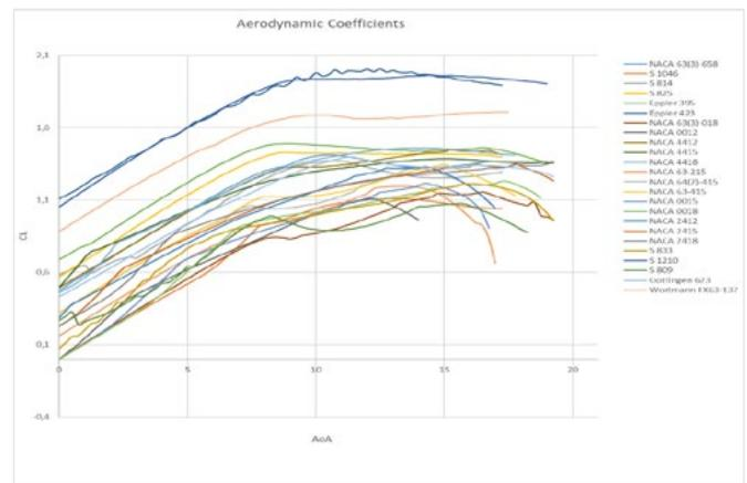
Figure 1.  $C_L$  values of the airfoils commonly used in horizontal axis Hydrokinetic Turbines.
