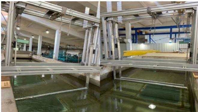
**Figure 5.** The Experiment Setup of the Single Cylinder (Left). The Experiment Setup of the Tandem Cylinders (Right)
