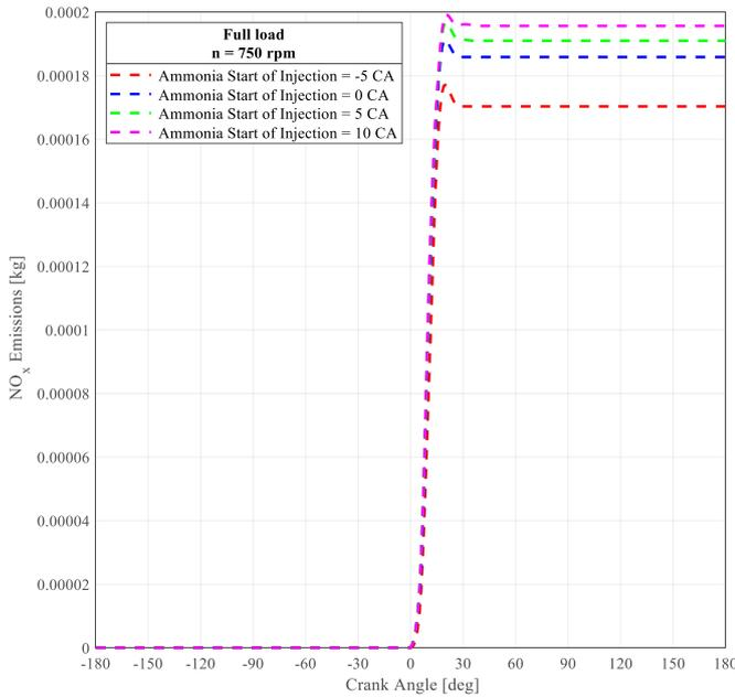
**Figure 2.** NO<sub>x</sub> emissions for different ammonia injection timing.
