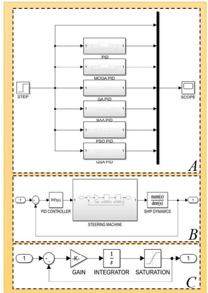
Figure 9. MATLAB/Simulink scheme of ship steering control system (A), MATLAB/Simulink scheme of ship steering control subsystem (B), MATLAB/Simulink scheme of ship steering machine subsystem (C).
