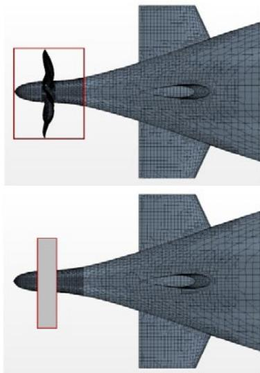
**Figure 6.** The gridding in stern area: the discretized propeller model (left); the body force model (right)
