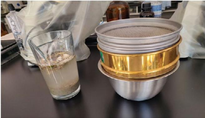
**Figure 9.** Sediment sample in saturated solution and sieve stack
