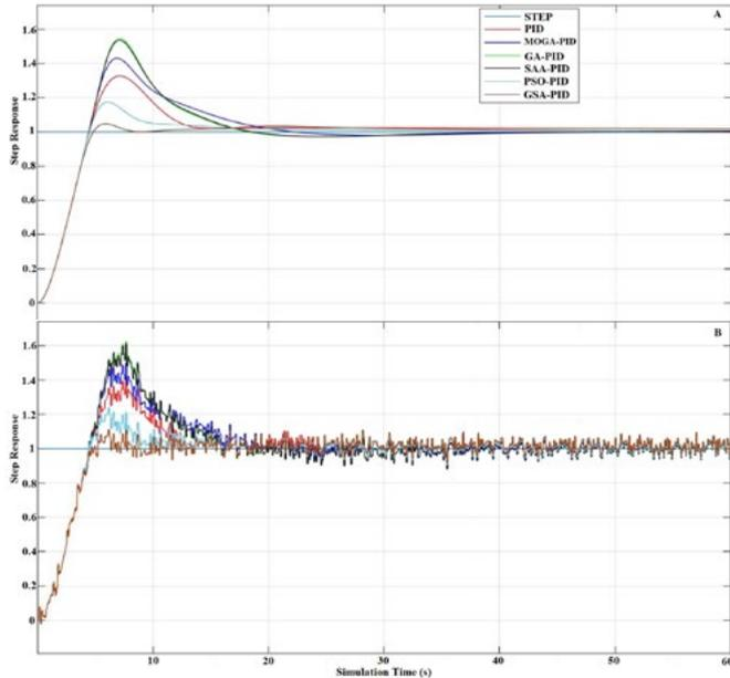
**Figure 10.** The simulation results of the study: step response of controllers (A), under the external factor effects (B).
