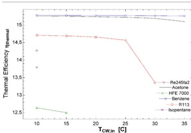
**Figure 3.** The effect of temperature of the sea water on the thermal efficiency of the ORC system for different working fluid types.
