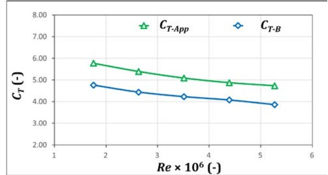
**Figure 7.** Comparison of bare and append resistance coefficient.
