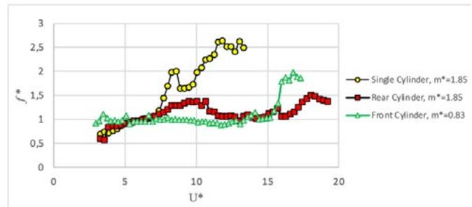
**Figure 10.** Comparison of Oscillation Frequencies of the Single Cylinder, Rear Cylinder, and Front Cylinder in Tests with Flow
