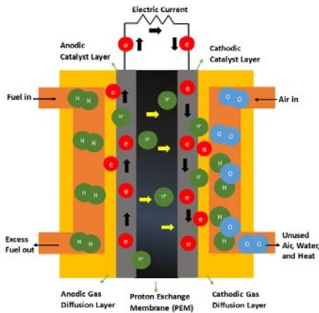
**Figure 2.** PEM Fuel Cell Working Principle [12]
