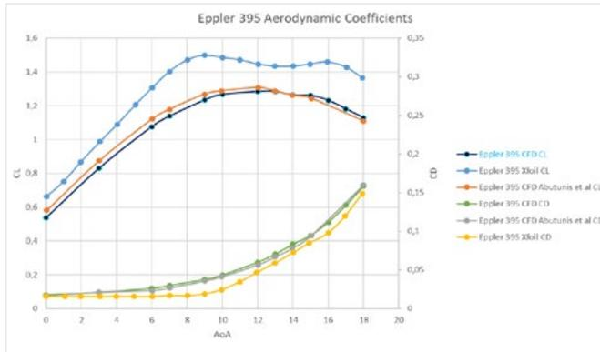
**Figure 8:**  $C_L$  and  $C_D$  values at different angles of attack ( $Re=1.65 \times 10^5$ ).
