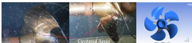
**Figure 6:** Case 2 Experiment and CFD Cavity Captures Comparison
