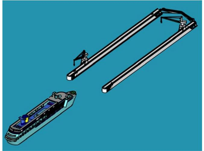
**Figure 10** Docking process in the floating platform
