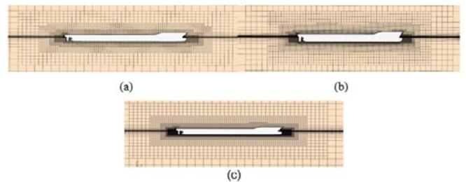
**Fig. 4** Grid structure (a) coarse, (b) medium, (c) fine
