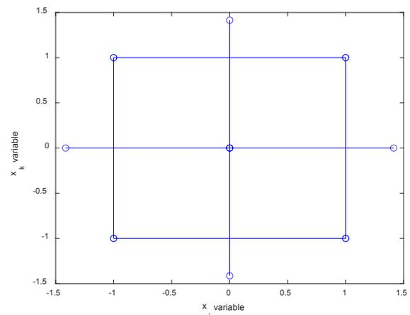
Figure 2. Central Composite Design for Design of Experiment
