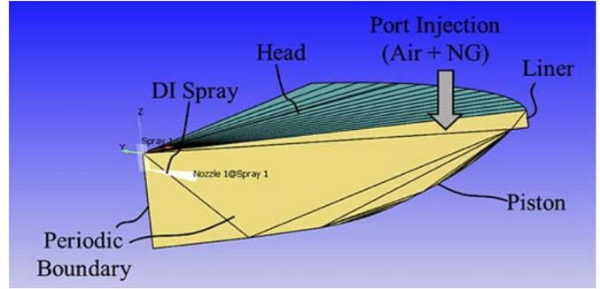
**Figure 1.** Computational domain of the RCCI engine with bathtub piston bowl at TDC.
