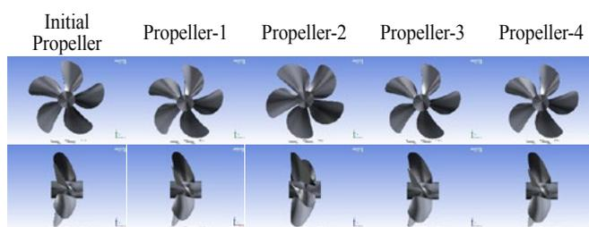
**Figure 8:** Parametrically Designed Propeller Geometries
