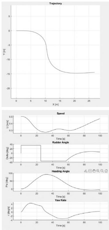
**Figure 4.** Course-changing & course keeping in ViL using PID. For demonstration purposes, the target heading angle has been chosen as  $0^\circ$  (corresponds to right in the figure) and  $k_p = 1, k_i = 0, k_d = 0$  has been used for the controller. The heading angle has been manually disrupted with a  $35^\circ$  rudder angle until  $t = 20s$ . At  $t = 20s$  the PID controller has been enabled
