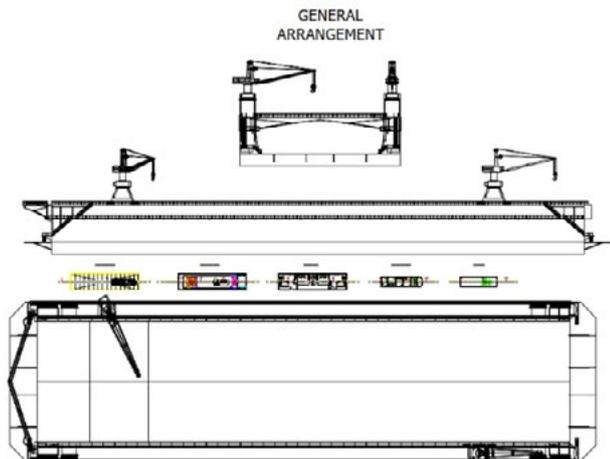
Figure 6 Floating platform general arrangement.
