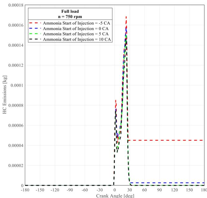
**Figure 3.** HC emissions for different ammonia injection timing.
