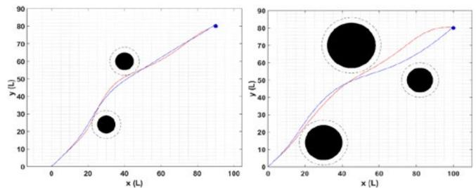
**Figure 8.** Simulation results for Map 1 (right) and Map 2 (left). Red line shows path with  $P=500$  and blue line shows path with  $P=1000$
