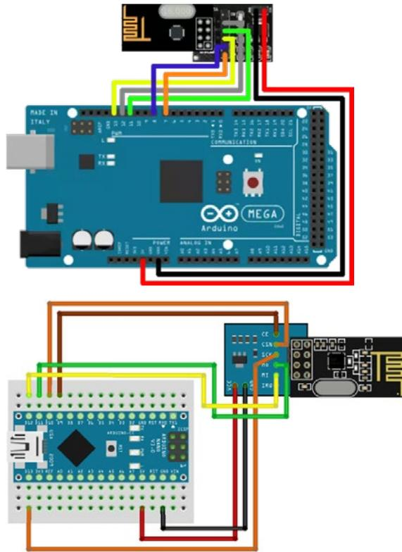
**Figure 6.** Transmitter and receiver circuit diagram
