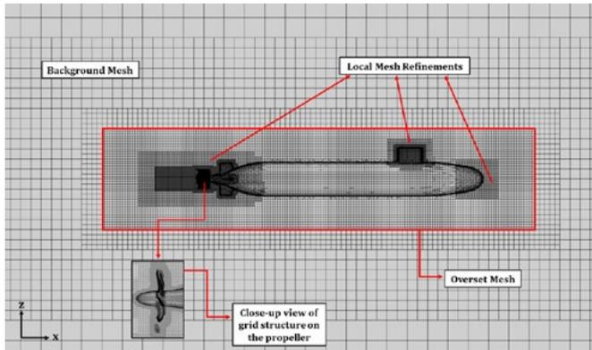
**Figure 5.** The overset mesh configuration in free-running simulations
