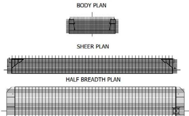
Figure 5 Floating platform linesplan
