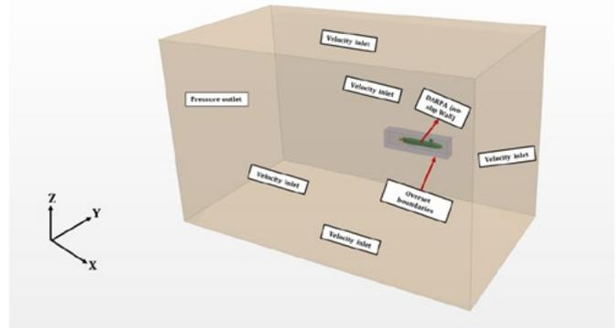
**Figure 3.** The solution domain and boundary conditions
