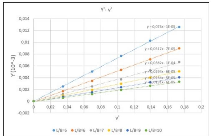
**Figure 15.** Dimensionless Coefficient Ratios (Lateral Drift Force and Yaw Moment).
