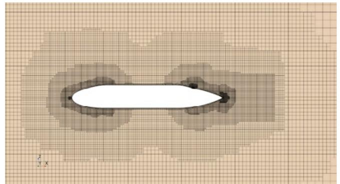
**Figure 3.** Unstructured surface and volume grid of the bare BB2 Joubert
