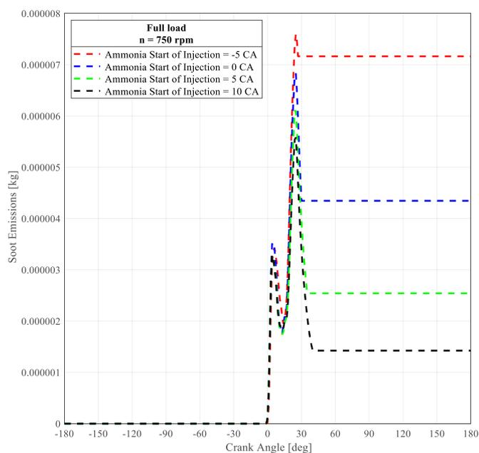
**Figure 6.** Soot emissions for different ammonia injection timing.
