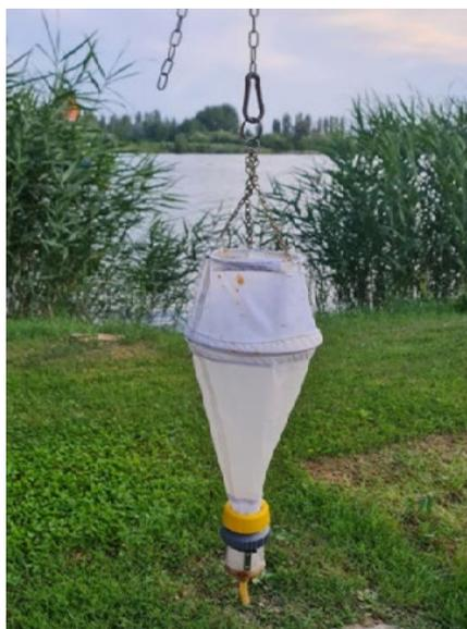
**Figure 2.** Plankton collecting net with a mesh size of 80  $\mu\text{m}$
