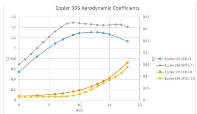
**Figure 7:**  $C_L$  and  $C_D$  values at different angles of attack ( $Re=2 \times 10^5$ ).
