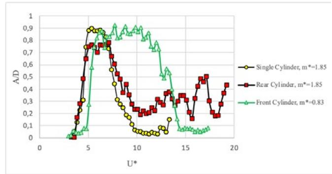
**Figure 9.** Comparison of Amplitude Responses of the Single Cylinder, Rear Cylinder, and Front Cylinder in Tests with Flow
