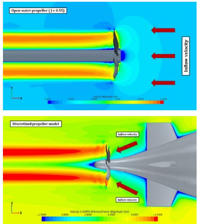
**Figure 11.** Comparison of the velocity distribution around the propeller: the open-water propeller case (above) and the free-running of the self-propelled submarine case (below)
