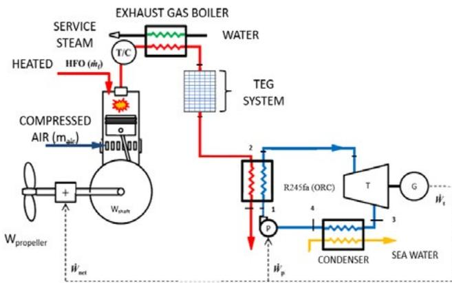
**Figure 1.** Example diagram when ORC and TEG are used together [28].
