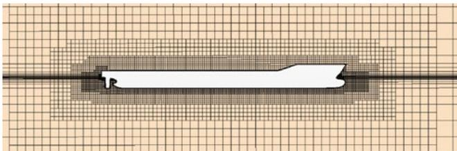
**Fig. 2** The grid structure around the KCS hull
