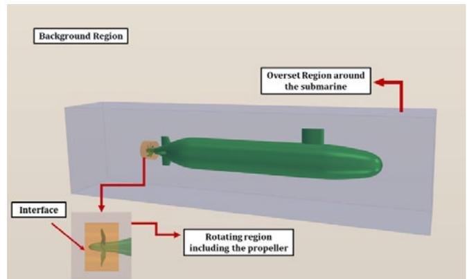
**Figure 4.** The details of the overset grid configuration
