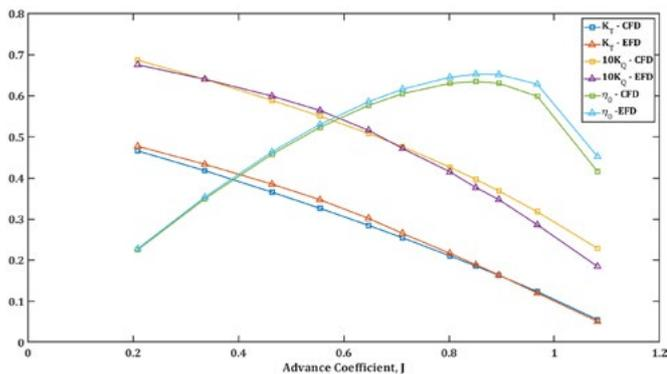
Figure 8. Validation of CFD results for open-water propeller tests
