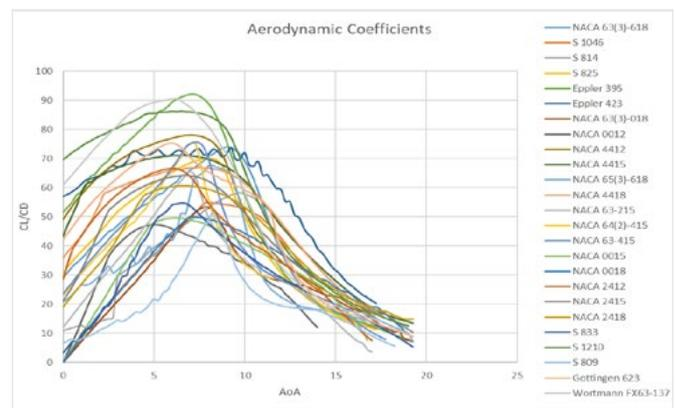
Figure 2.  $C_L/C_D$  values of the airfoils commonly used in horizontal axis Hydrokinetic Turbines.
