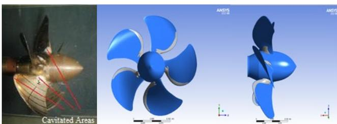
**Figure 7:** Case 3 Experiment and CFD Cavity Captures Comparison
