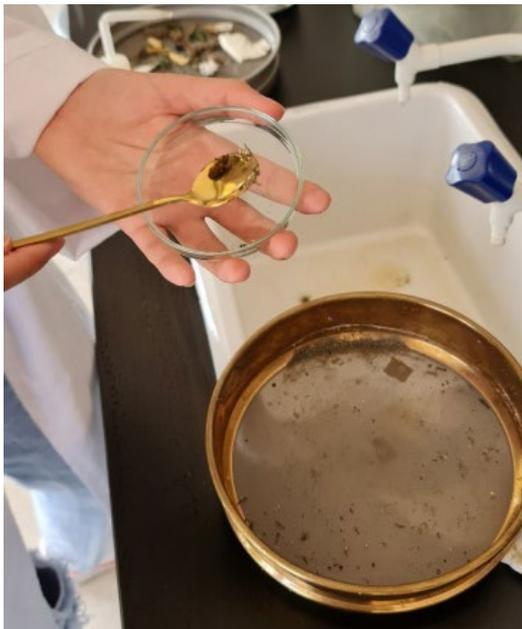
**Figure 4.** Transfer of sieved sample for further sorting and analysis
