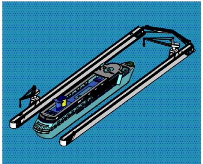
**Figure 11** Ship entering floating platform and sitting on the blocks
