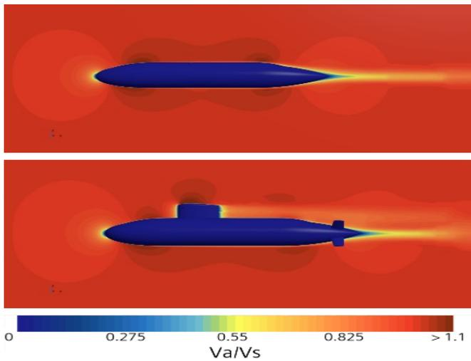
**Figure 8.** Velocity distributions around the bare hull (top) and the fully appended hull (bottom) for  $V=2$  m/s.
