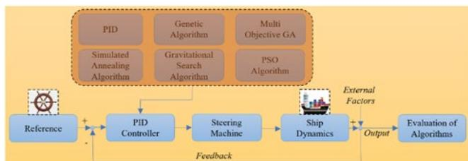
Figure 8. The methodology of the ship steering system PID coefficients' optimization process.
