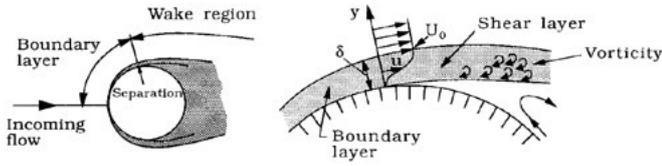
**Figure 1.** Schematically Representation of Boundary Layer and Wake Region [3].
