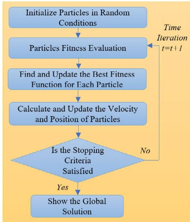
**Figure 5.** Flowchart of the Particle Swarm Optimization Algorithm
