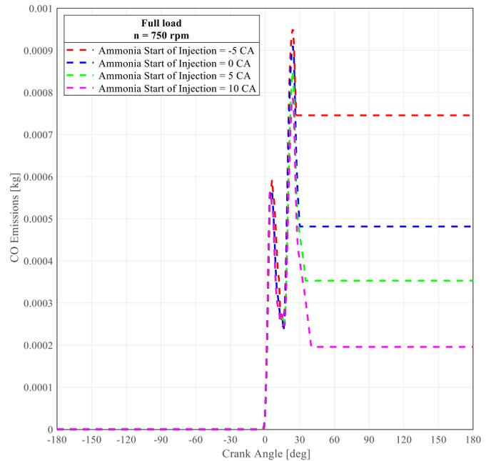
**Figure 4.** CO emissions for different ammonia injection timing.
