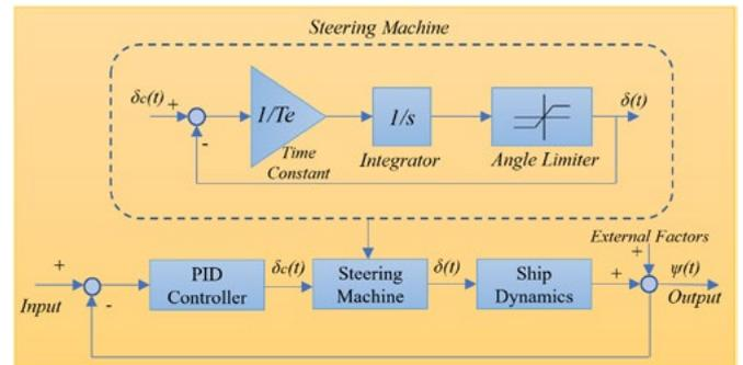
**Figure 2.** Block diagram of the steering system and machine.
