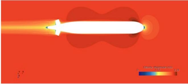
Figure 9. Velocity Distribution at 2 m/s.
