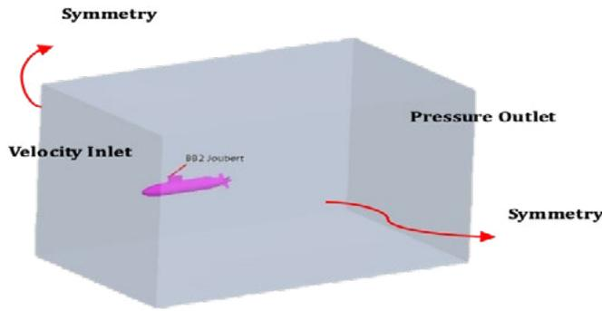
**Figure 1.** Computational domain with boundary conditions
