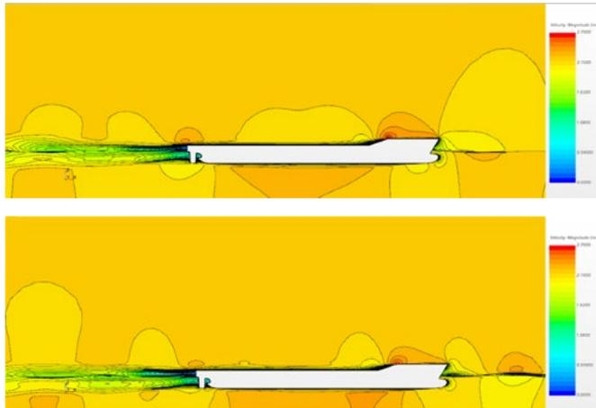
**Fig. 8** Velocity profile around the ship in shallow water ((upper:  $H=5T$ , lower:  $H=3T$ ))
