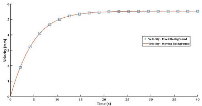
Figure 9. Comparison of the effect of the domain type on the submarine velocity
