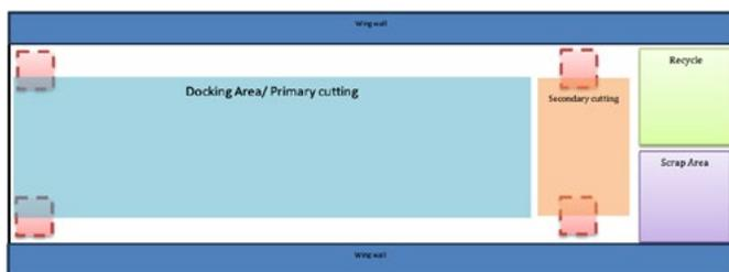
**Figure 4** Layout design of floating platform for ship recycling
