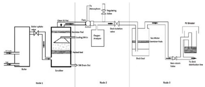
**Figure 1.** Inert gas system diagram with operating points.
