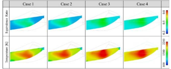
**Figure 3.** In-cylinder temperature and equivalence ratio distribution for four cases at +10° aTDC.
