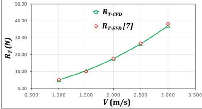
**Figure 5.** Comparison of CFD and EFD results for fully appended Joubert BB2.
