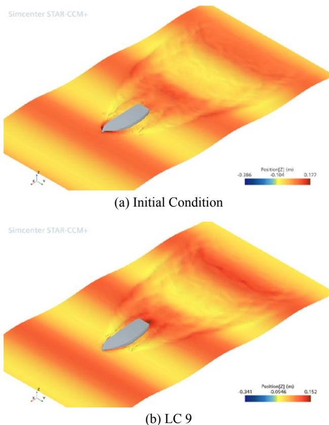
**Figure 5.** The result of CFD seakeeping simulation at  $\lambda/L_{bp} = 2$
