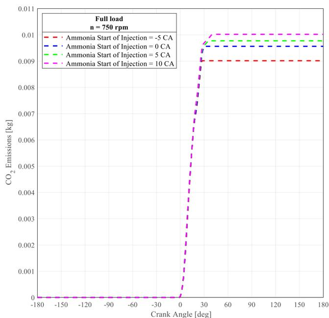
**Figure 5.** CO<sub>2</sub> emissions for different ammonia injection timing.
