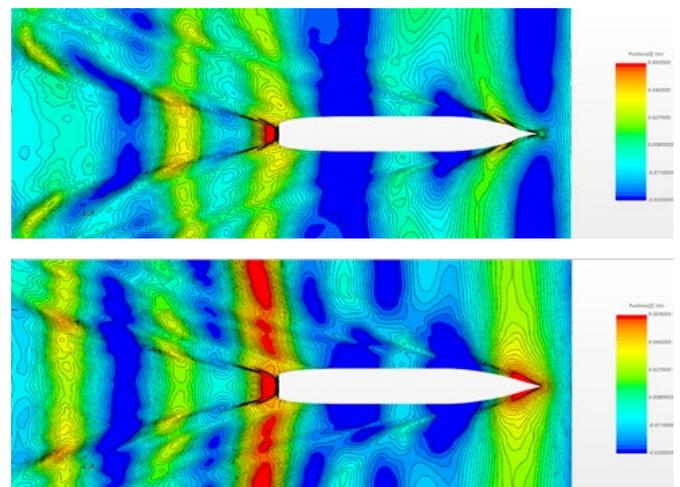
**Fig. 7** Free-surface profile for (upper: H=5T, lower: H=3T)
