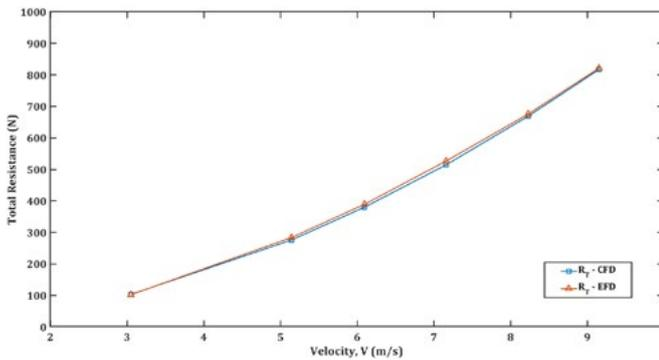
Figure 7. Validation of CFD results for submarine total resistance
