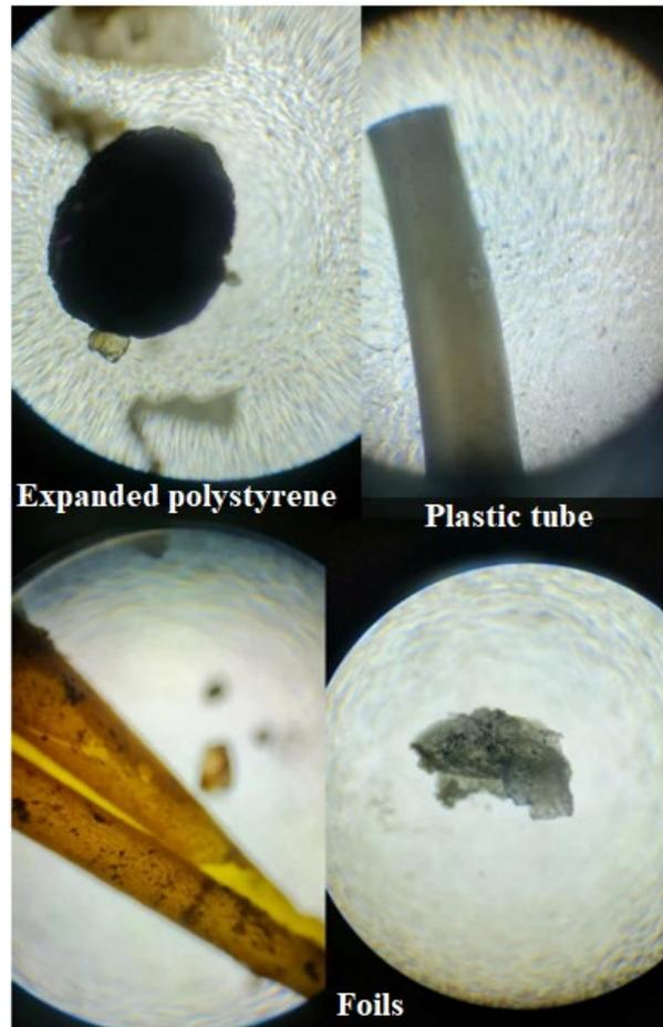
**Figure 12.** Micro-plastic identification under the microscope
