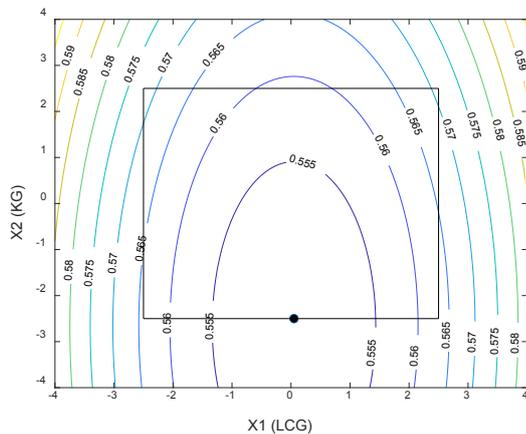
**Figure 3.** Response Surface Result for  $R_y$  Influenced by LCG and KG with the constrains and optimal location
