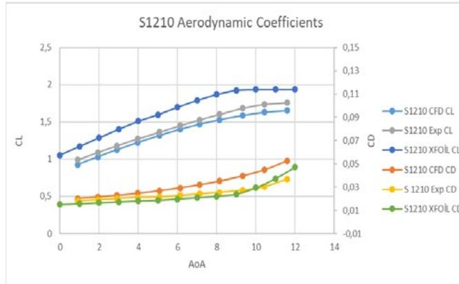
**Figure 5:**  $C_L$  and  $C_D$  values at different angles of attack ( $Re=2 \times 10^5$ ).
