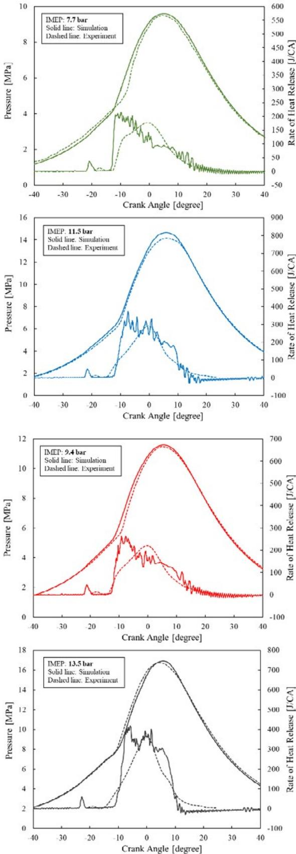
**Figure 2.** Comparison of experiment and simulation cylinder-averaged pressure traces.
