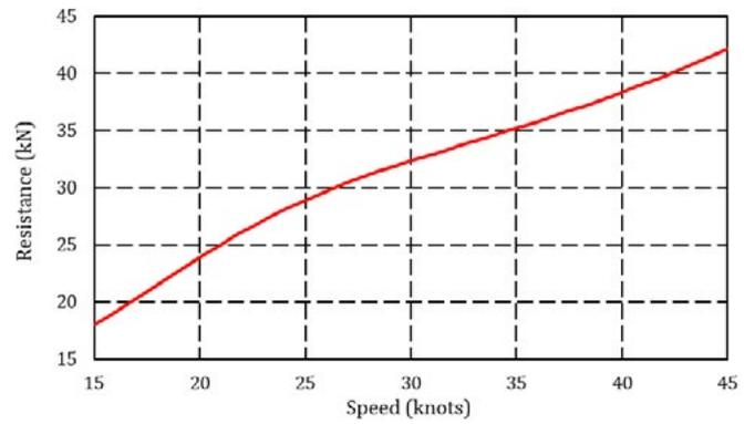
**Figure 9.** Resistance-Speed Diagram
