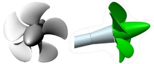
**Figure 2:** VP 1304 CAD Model [9]
