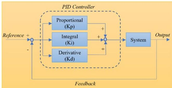
Figure 3. Basic concept of the PID controller
