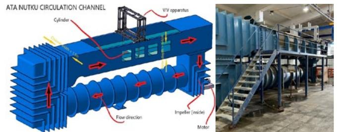
**Figure 4.** The CAD View of the VIV Prototype System (Left) (8). The Circulation Channel in Ata Nutku Ship Model Testing Laboratory (Right)
