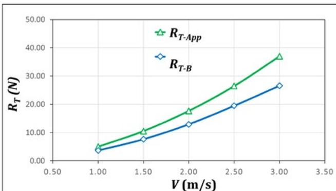
**Figure 6.** Comparison of bare and append resistance results.
