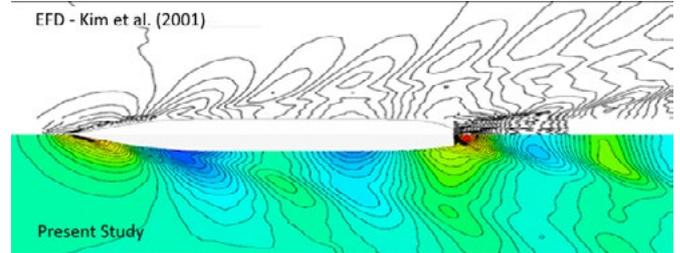
**Fig. 6** Comparisons of wave pattern for EFD (top), CFD (bottom)
