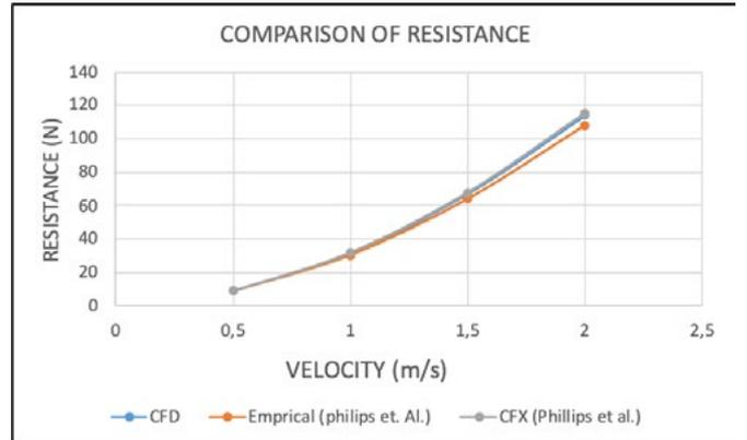
**Figure 7.** Comparison of Experimental and Analytical Data of the Autosub Vehicle.
