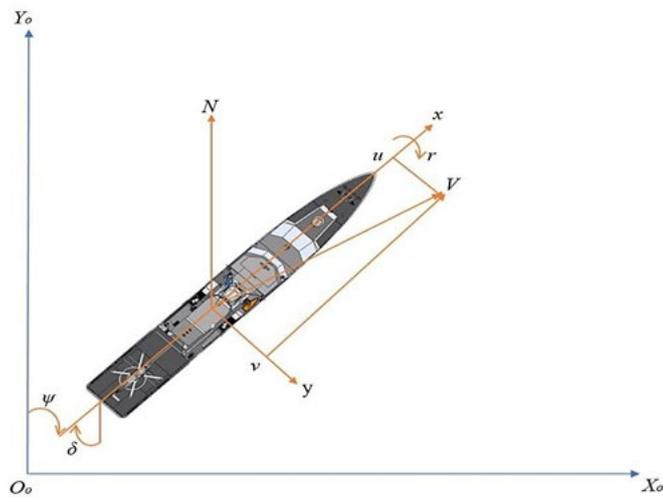
**Figure 1.** Ship motion components.
