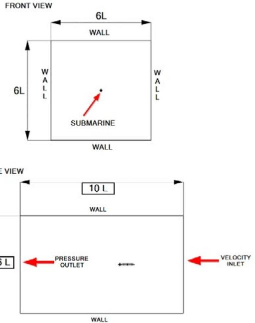
**Figure 3.** Boundary Conditions for Static Drift Analysis.
