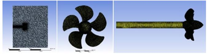
Figure 4: Mesh View of PPTC VP 1304 Propeller
